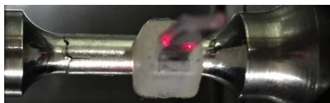
Figure 5 Example of photo image of a crack generated in the specimen
