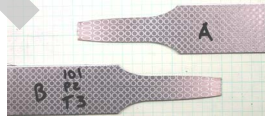
FIGURE 6 - PULSED SPECIMEN WITH DIFFUSED NECK
