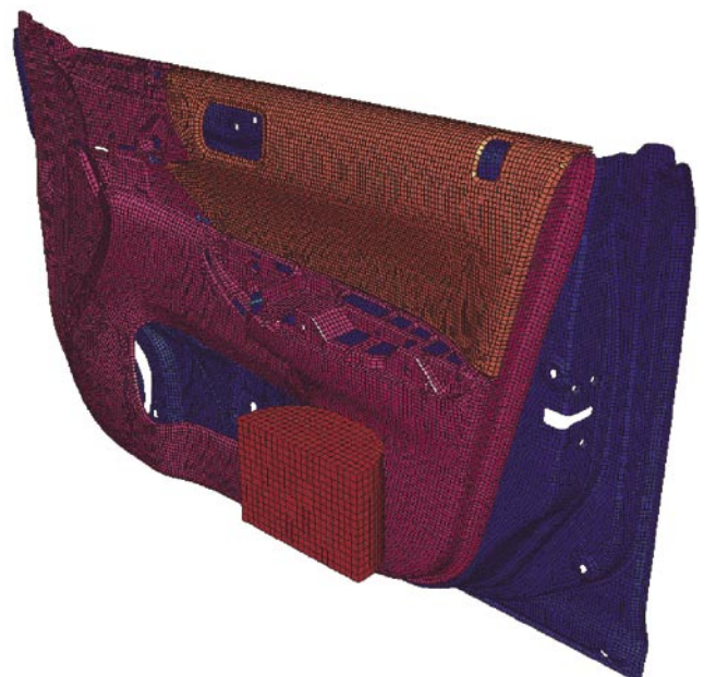
Fig.2 Finite Element Model of Door Trim Impact Test
