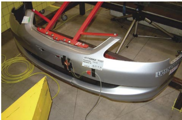
Fig.3 Photograph of Bumper Face Impact Test
